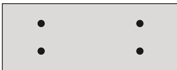
2-Drill little holes corresponding to the vertices
