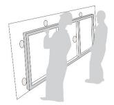
The use of suction cups is an ideal way of moving slabs manually. Large pieces, particularly those that are long and narrow, may require the use of aluminum spreader bars in addition to the suction cups to prevent the slab from bending.
