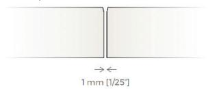
Porcelain slab seams should <u>NOT</u> be polished or "flattened" with a grinder. Doing so will create a noticeable difference in the surface finish at the seam when compared to the rest of the slab(s).
