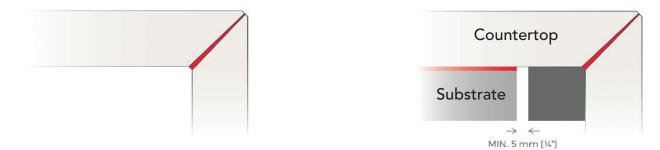
For all installations, be sure to leave a ¼" gap between the miter support block and the countertop substrate. This will allow for differences in thermal expansion between the two surfaces.
