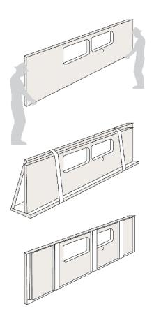
Transport both raw and fabricated Della Terra<sup>®</sup> Porcelain Slabs vertically, using wooden crates or A-frames to protect the slabs from damage. Place foam or polystyrene inside crates to protect slab edges. When using an A-frame, it is important that the slabs are fully supported with an appropriate backer, and that the edges are securely clamped to prevent vibration.
